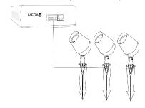
**DECO DRIVE CV3 DIN** (One unit per output port, up to 3 when power linked. Total of 3 outputs x 9 fixtures.)
