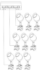
**DECO DRIVE CV4** (One unit per output port, up to 3 when power linked. Total of 4 outputs x 12 fixtures.)
