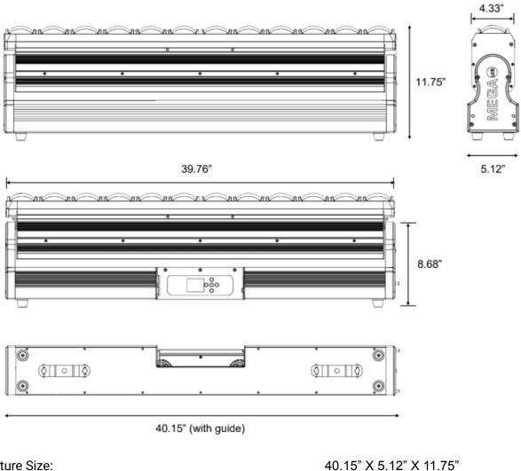
Fixture Size: Fixture Weight: Packaged Size: Packaged Weight:
