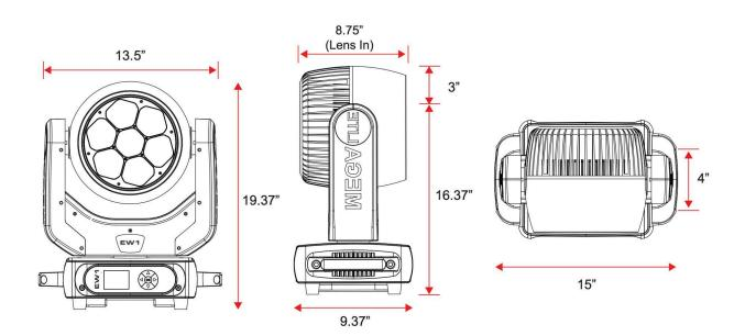
Fixture Size: Fixture Weight: Packaged Size: Packaged Weight: 15" X 9.37" X 19.37" 32lb 16.5" X 13.5" X 24.5" 35.25lb
